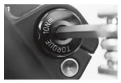
1. Slide in the axle and tighten it with a 6mm Allen wrench by suggested tightening torque of 10Nm.
