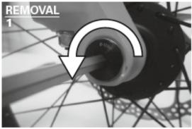
Loosen the axle on the drive side with a 6mm (15AH2) or 5mm (12AH2) .
