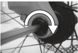
2. Tighten the axle with a 6mm (15AH2) or 5mm (12AH2) Allen wrench by the suggested tightening torque of 8-10Nm.
