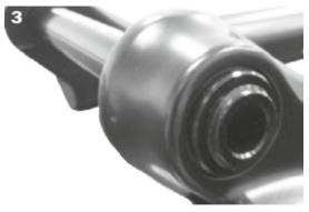
3. Check the axle's thread. It must be visible.
